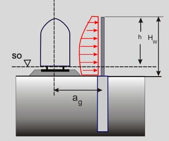
Alternating pressure and suction forces due to passing train main cause fatigue effect
