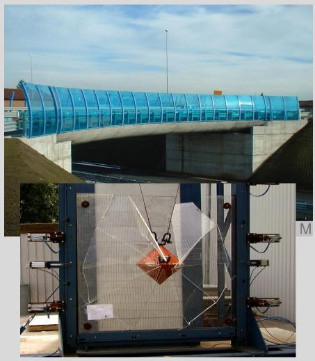
Risk from falling debris may occur in case of noise barrier installed on bridges or critical positions – (EN 1794-2)
